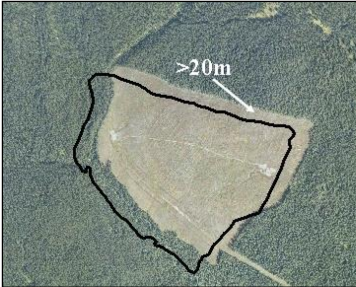
Figure 14 Relative positional accuracy overlay. This polygon is greater than 20 m from its true location. This submission would fail.
